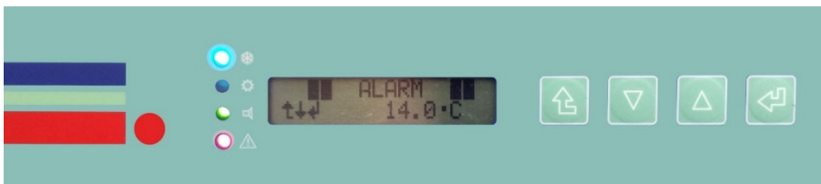
Example Temperature Alarm Display, high of 14.0°C reached
