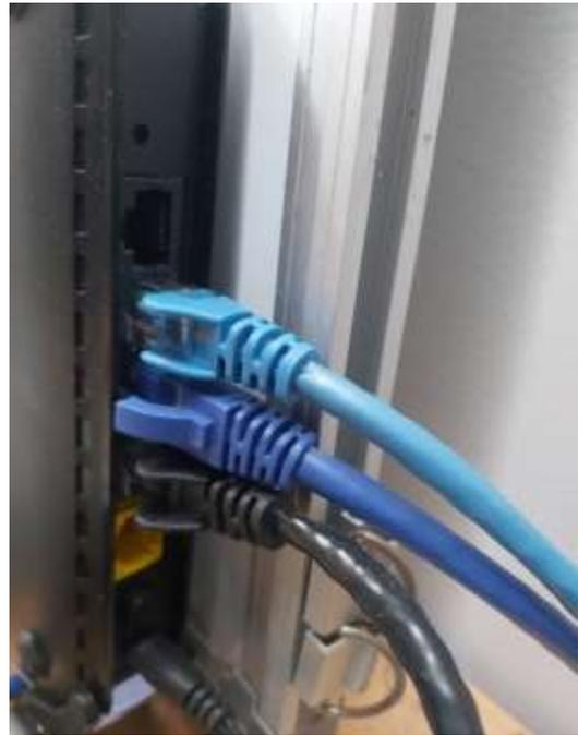
6. Connect the power cable and network cable to the back of the wireless base station and then switch on.
