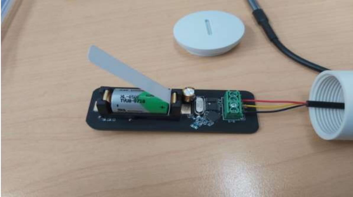
3. Pull the white plastic battery tab out. It may be easier to remove the battery completely and then replace. Take note of which way the battery is to be inserted (**Positive points to the wires**).
