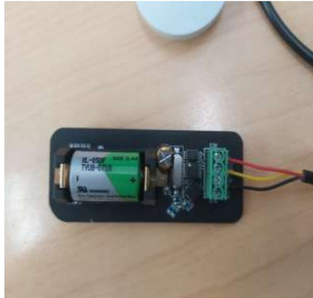
4. Slide the circuit board back into the white tube and replace / tighten both end caps. **The sensor is now ready to go.**
