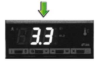
The current set point for the fridge can be checked by pressing and holding the "I" button. This set point is showing  $3.3^{\circ}$ C. This will typically show around  $3.0^{\circ}$ C. This can be adjusted by pressing and holding the "I" button and using the " $\mathbf{V}$ " and " $\mathbf{A}$ " buttons to suit.
