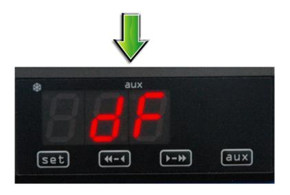
By holding " $\blacktriangleleft \blacklozenge \dashv$  " and " $\triangleright \lor \triangleright \triangleright$ " buttons together this forces the fridge into defrost mode for the programmed time and will then continue its normal operation.
