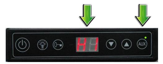
If the high alarm is going off it may be from the door being open or a power cut if one has occurred.
