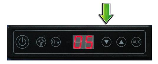
To reset the recorded high and low temperatures in memory, **press and hold** either of the temperature buttons and then press and hold the other temperature button simultaneously for 3 seconds until you hear a  $2^{nd}$  beep.
