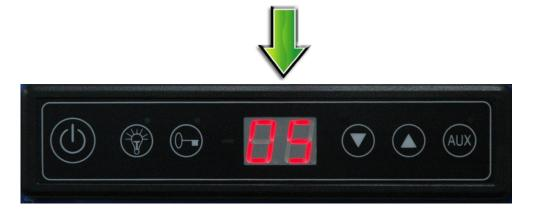
This button is to check the low temperature. Press the button to display the lowest recorded temperature since the controller was last reset. This low temperature is reading -2°
